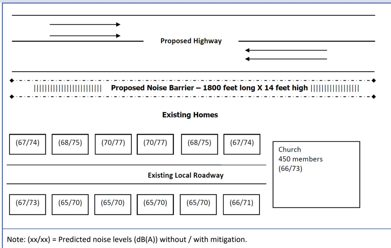
**SCENARIO FEATURES.** The twelve (12) single-family homes each represent 1 receptor. The twelve (12) single-family homes were not built prior to the roadway. To complete the analysis for this scenario, however the ER must be calculated for the church.
