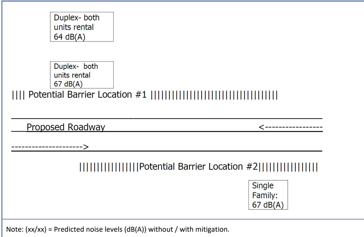
**SCENARIO FEATURES.** The single-unit resident on the south side of the roadway represents one (1) receptor, is a front-row receptor, and is an impacted receptor. On the north side of the roadway, both duplexes represent two (2) receptors for a total of four (4) receptors. One duplex is considered a front-row receptor. Only one of the duplexes approaches or exceeds the NAC for Activity Category B, so there are two (2) impacted receptors north of the proposed roadway.
