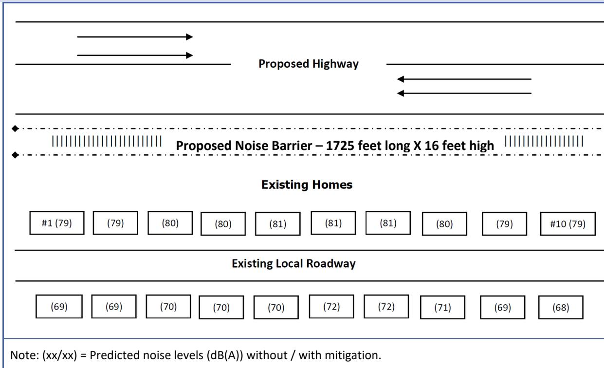
**SCENARIO FEATURES.** All single-family residences represent one receptor, so there are twenty (20) receptors in this scenario. All twenty (20) receptors were built prior to proposed highway. Ten (10) of the receptors are considered front-row receptors. All twenty (20) receptors in this scenario exceed the NAC for Activity Category B.
